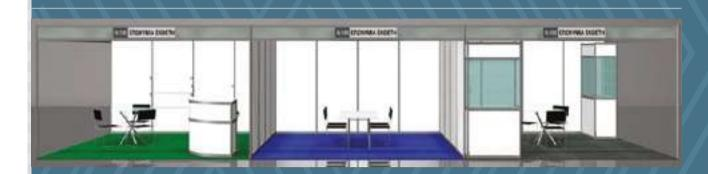
The 2.50 m-height standard stand, is made of a natural coloured aluminum frame, with white-coloured PVC panels (OCTANORM).
